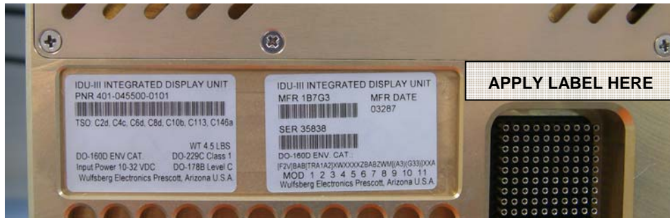
Figure 10 Typical DO-178B Level A Label Location
